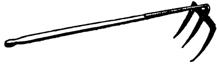
No. 1.—Length of handle, including iron socket, 4 feet 9 inches; diameter of handle, 1½ inch; width of the head, 6½ inches; length of curved teeth, or prongs, 6½ inches.
